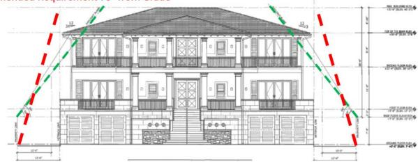
In the second example below, the house is required to be elevated approximately 6 ft. above its surrounding established grade in order to meet FEMA and Town floodplain elevation requirements. The green dashed line shows the Daylight Plane requirement, for a 60 ft. wide lot (with a current 62° degree angle required), applied from the Design Flood Elevation. The red line shows the proposed requirement of a 75° degree Daylight Plane angle, measured from established grade.
