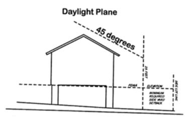
The City of Sarasota's Daylight Plane requirements for single-family structures (typical maximum single family zoning heights are 35 ft.) is very similar, with a 45 degree slope of no-development generally measured from the minimum required side lot line setback, and beginning at 25 feet above the FEMA required elevation. See graphic below.
