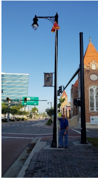
Manatee County Downtown Bradenton ~25-ft. poles with ~4-ft. arms Pole diameter of ~ 8 inches Base diameter 16 inches
